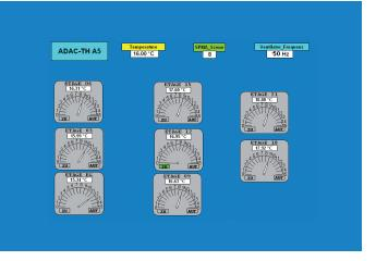
Fig. 6: Overview of the temperatures on the individual floors, outside temperature and setting of the damper motors for supply of air to the stairwell.
