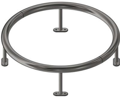
Anti-ram-guard made of 50 mm diameter stainless steel tube. Outer diameter 816 mm, height 235 mm.
