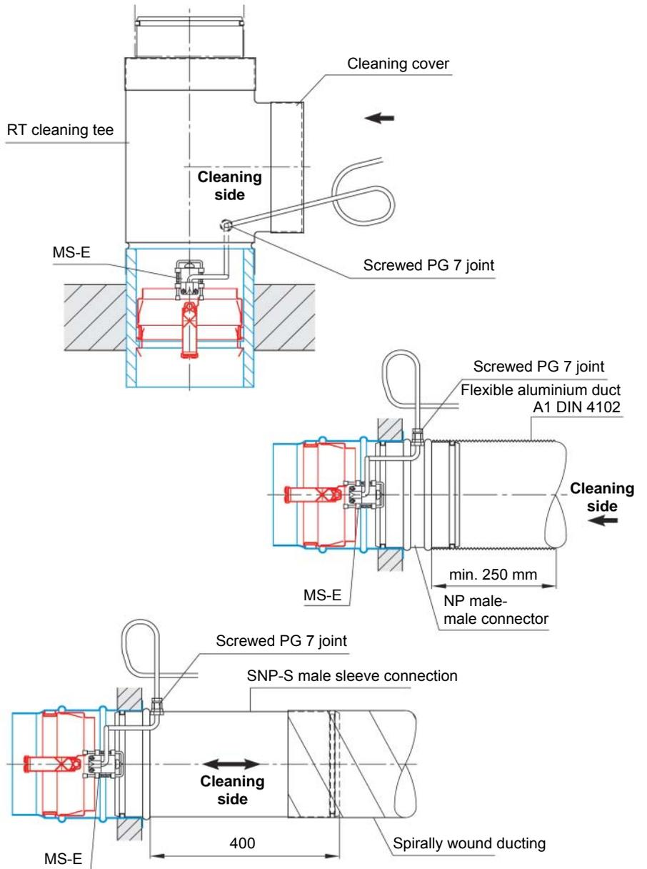
Lead the cable of the MS-E limit switch out of the screwed joint (PG 7) and leave a loop of ca. 50 cm with a cable binder outside the duct for inspection, so that the damper can be removed easily
