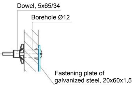
For mounting within shaft walls that are min. 24-34 mm thick, not embedded with mortar
