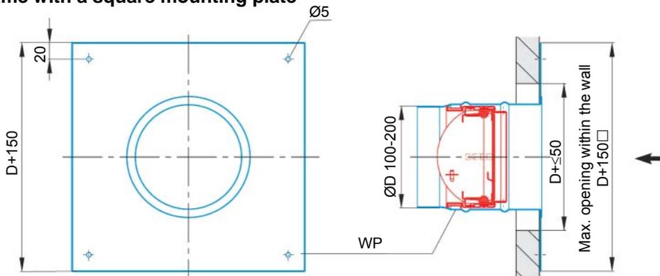
**WP-Z mounting frame with a square mounting plate for installing flush with the shaft**
