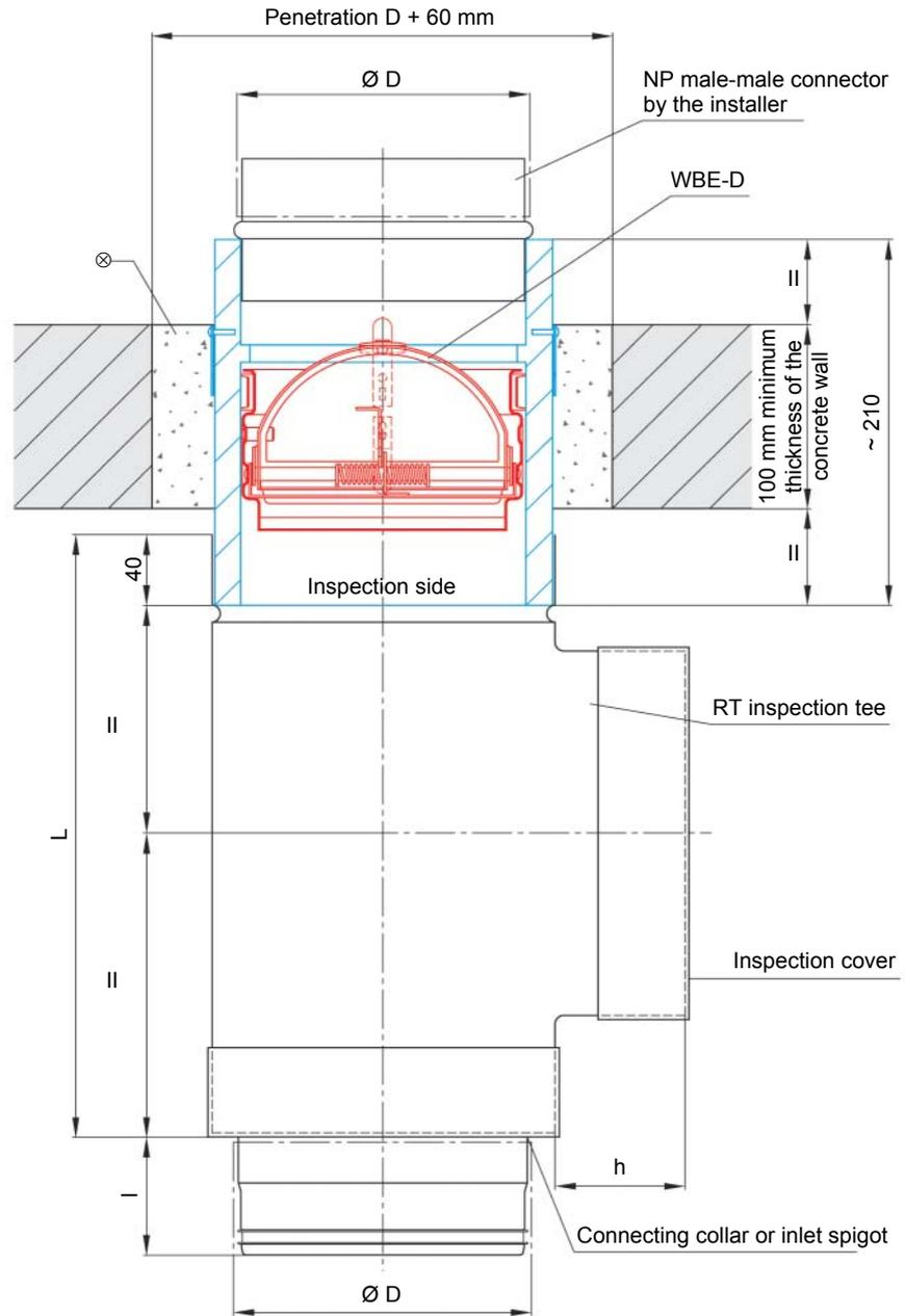
⊗ Surrounding gap filled with mortar, mortar group II or III, DIN 1053 or with gypsum
