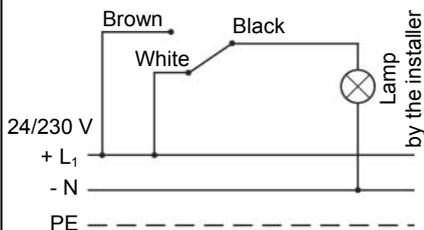
**Facility to inspect the WBE-D damper including electrical limit switch**
