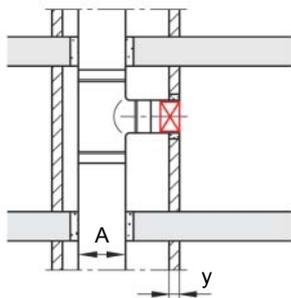
Installation outside of a service shaft with internal fire load\*
