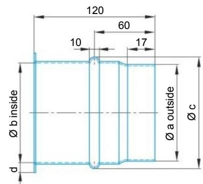
**Special mounting frame (only in NW 100) for the direct connection to a sound-absorbing bend**
