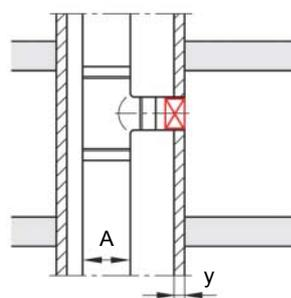
Installation outside of a service shaft without combustible materials
