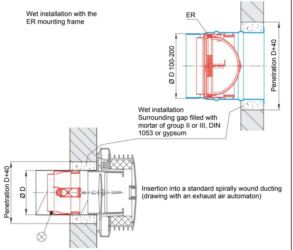
**Installation inside of F90/F30 shaft partition walls, L90/L30 classified or system-tested shaft with a mortar embedding (WET INSTALLATION)**
