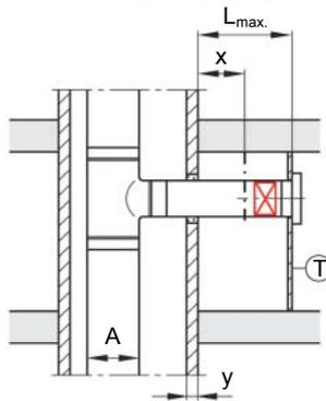
Installation inside and outside of classified service shafts (with combustible materials, e.g. electric cables or plastic ducts)
